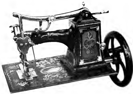
Figure 95.—[A.C.]HERRON'S PATENT SEWING MACHINE, 1858. The manufacturer of this machine is not known, but the machine was based on the patent of Abial C. Herron issued August 4, 1857. All the machines carry a small heart-shaped plate just above the needle descent bearing the patentee's name and the patent date. The patent covered an improvement in the method of making the chainstitch. The machines were provided with a hand crank, but were also meant to be operated by a belt and treadle. No records of the extent of manufacture of this machine have been found. This machine head measures 14 inches in width, about standard size. (Smithsonian photo 48329-J.)
